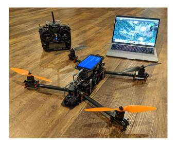
FIGURE 16. DRONE ASSEMBLY WITH MOBILE DEVICE
