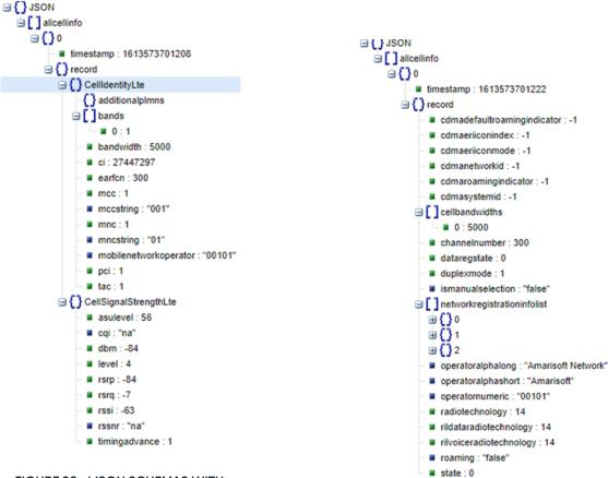
FIGURE 20. JJSON SCHEMAS WITH SAMPLE DATA FOR "CELLIDENTITYLTE" AND"CELLSIGNALSTRENGTHLTE" RECORDS
