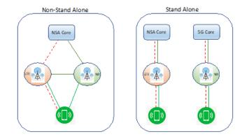
FIGURE 3. 5G NETWORK DEPLOYMENTS, ILLUSTRATING STANDALONE VS. NON-STAND-ALONE (NSA) ARCHITECTURE
